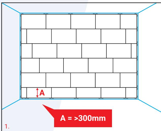
**It is critical that the first row is laid accurately. If it is not straight the floor will be out of alignment.**
