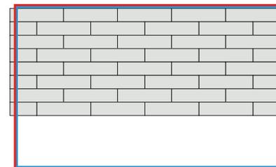
If the cut of the last panel of the first row is too small (less than 300mm), cut a new panel in half and start the next row with this half-panel.
