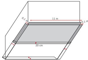
Lay the damp-proof membrane onto the sub-floor and unfold it, ensuring there is 100mm along the length and both ends are folded against the wall.
