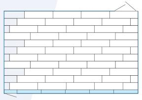
If the cut off panel is less than 300mm long use a new full panel to start the next row. Carefully measure the Lay the cut panel with the pry bar. and the wall (allow for the 10mm spacer blocks, or optional plastazote strip).
