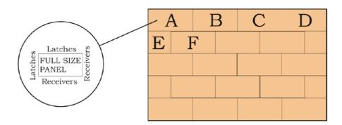
Lay the first row of panels along the length of the room, but DO NOT latch the panels together at this stage (panels A-D on diagram).
